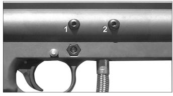
To release the power tube and valve, unscrew the two valve bolts on the outer right-side receiver.
