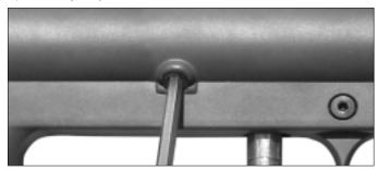
To adjust the velocity use the 5/32" allen wrench included with your gun. The velocity adjustment screw is located on left side receiver at a 45° angle. To adjust the velocity down, turn the screw inward or clockwise. To turn the velocity up, turn the screw out or counterclockwise (*Do not remove velocity screw*).
