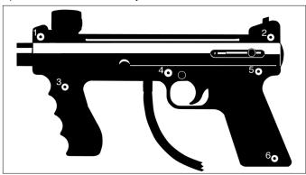
To remove the left-side receiver, unscrew all (6) receiver connection bolts. Then carefully lift the left-side receiver to access the internals.
